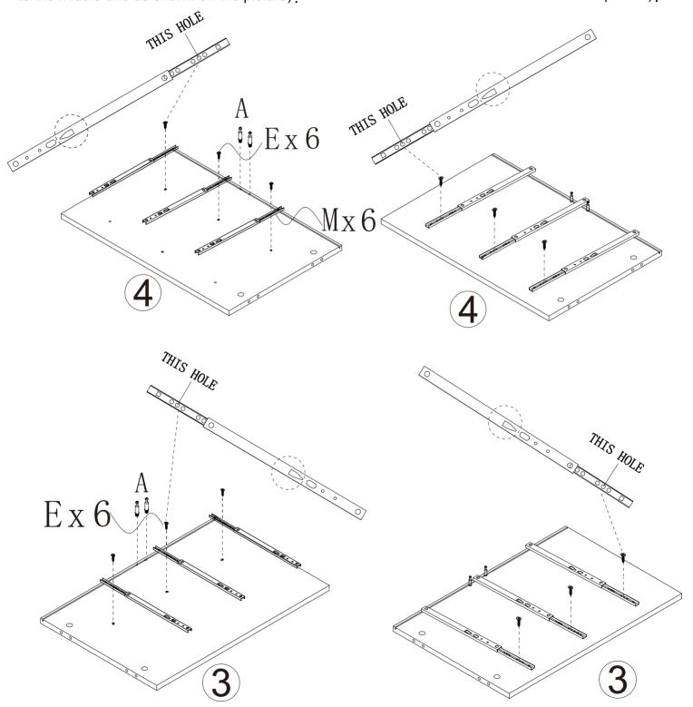
Stretch Hardware M and fix it to Panel 4&3 with screw E.
