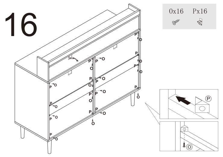
Lock Hardware P at 16 corners of backboard with O.
