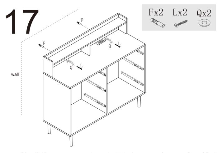
If it is a solid wall, please use expansion and self-tapping screws to secure the cabinet to the wall, if it is a wooden wall, only use self-tapping screws, please do not overtighten the screws.
