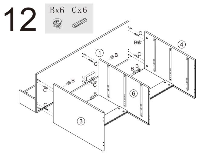
Lock Panel 1 to 3&6&4 with Hardware C&A&B(C/A first).
