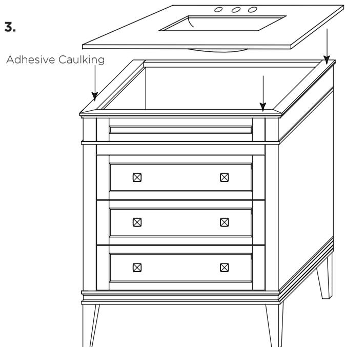
**STEP 3:** Secure top & back splash to cabinet by using adhesive caulk
