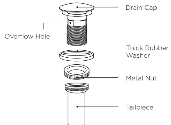
**STEP 3:** From under the drain, insert the thick rubber washer and screw on and tighten the metal nut. Remove excess plumbers' putty.
