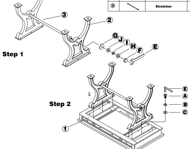
NOTE: DO NOT TIGHTEN ALL THE BOLTS UNTIL THEY ARE INSTALLED IN CORRESPONDING HOLES!
