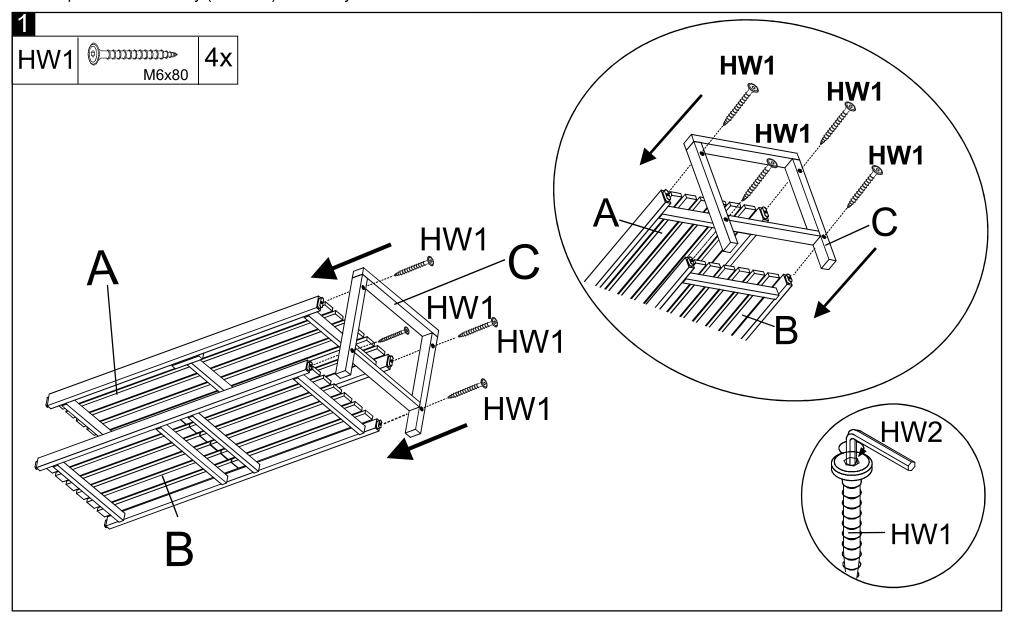
Step 1: Attach the Side (C) to the Seat (A) and the Tray (B) as shown on the picture . Using the Allen screw (HW1) to fix the Side (C) to the Seat (A), the Tray (B) by the Allen key (HW2).
