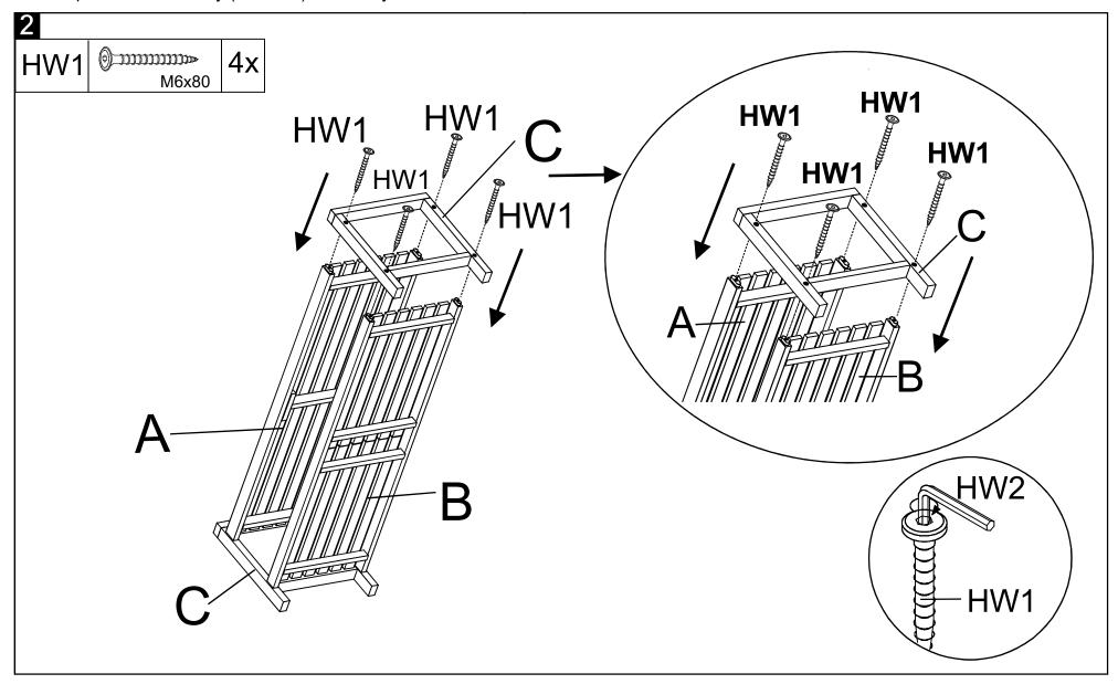
Step 2: Attach the Side (C) to the Seat (A) and the Tray (B) as shown on the picture . Using the Allen screw (HW1) to fix the Side (C) to the Seat (A), the Tray (B) by the Allen key (HW2).
