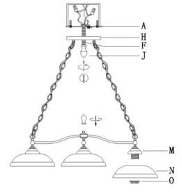
8) Install bulbs (Not included). Please do not exceed the maximum wattage capacity recommended on the socket.
