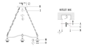
5) If needed, cut off the wires length of fixture. At this point, the remaining wire length measured from the top center of canopy (H) is at least 6".
