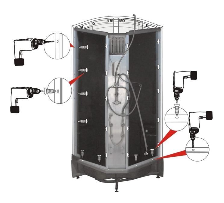
Place the shower rooftop onto the back glass panels and upper rail, securing using 3 self tapping screws into each panel. At this time connect all electrical conections by matching the labels with their appropriate spot. Also take the time to securely connect water accessories such as the hand shower, foot massager and shower head.
