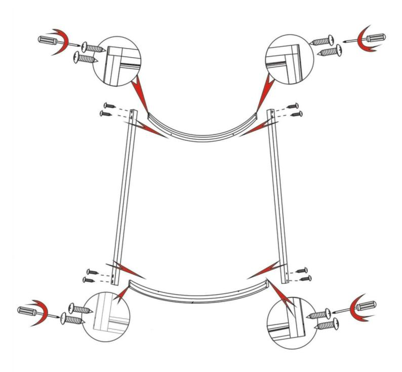
Fit the rubber gaskets on each long side of each side glass. Use a rubber mallet to gently tap the gaskets onto the glass if needed. Repeat those steps for the opposite edges of the side glass. Place the front columns vertically in between the upper and lower rails secured by screws.
