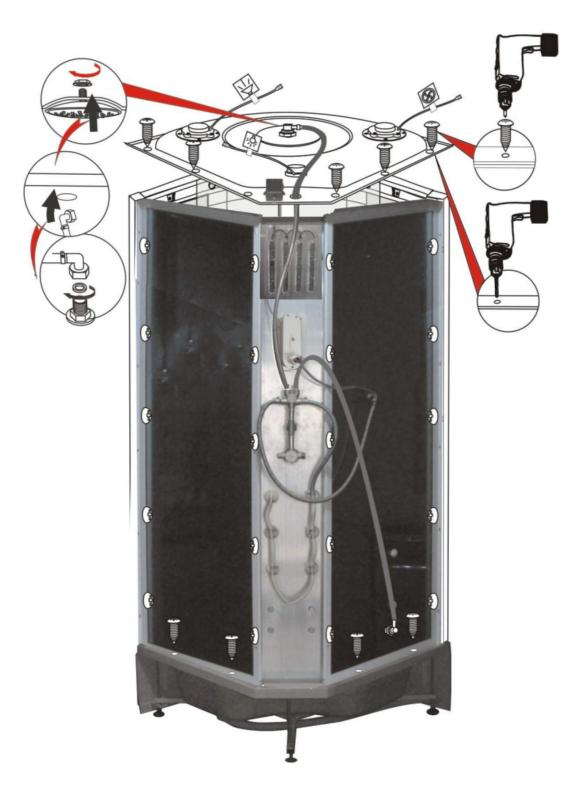
Hook up the shower's cold and hot water hoses to the home's cold and hot water hookups. Connect the shower to power ensuring that the correct electrical requirments of 30 amp GFCI breaker, 110 volts, 10 guage wire are met.
