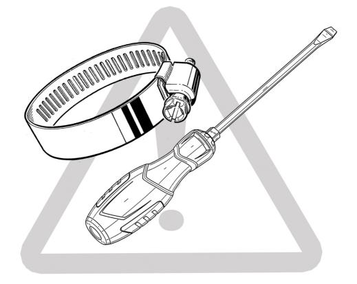
Please ensure all hose clamps are tightened before running any water through, failure to do so could result in water leaking. Make sure all connections and fittings are secure
