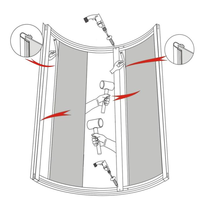
Install door handles to each door by placing the handle side on the outer part of the door and the screws on the inner part of the door. Door seals can be placed on the outer edge of the glass doors, slightly tap them in with a mallet. Magnetic door strips must be placed on the inner edge of the glass doors where the doors meet. A rubber mallet may be used to slightly tap them in as well.
