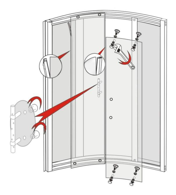
Attach the door rollers through the two top and bottom holes found on the glass doors. Use a wrench to adjust the height of the wheels to ensure a smooth gliding motion when the door opens and closes.
