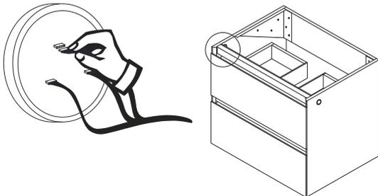
**STEP2.** Push out the switch button from inside with a screw driver gently
