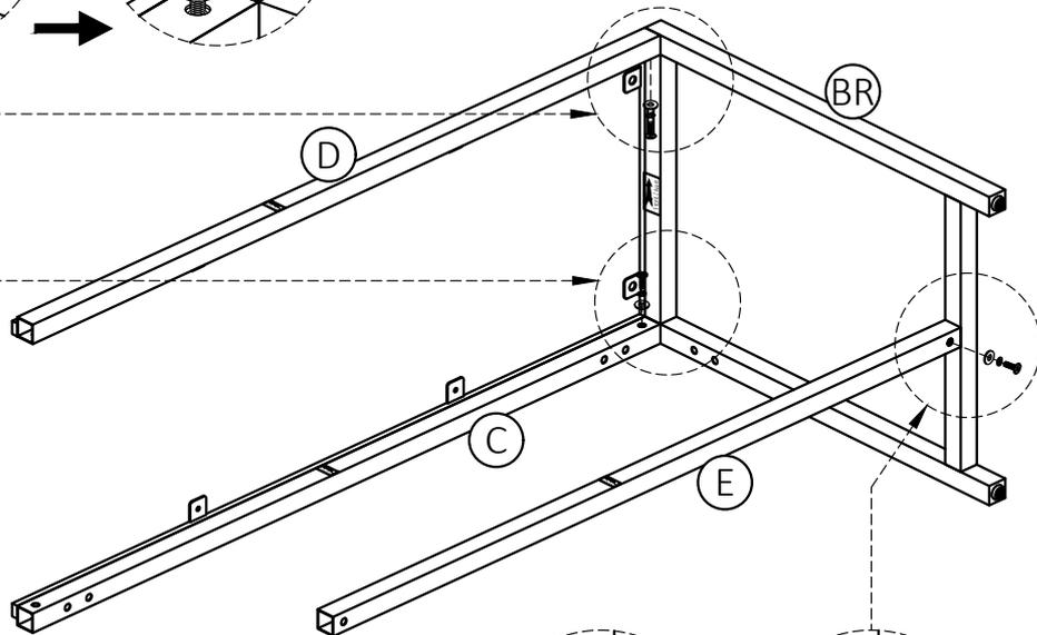
2. Use one Bolt (1), one Lock Washer (2) and one Washer (3) to secure each part (C), (D), (E) with (BR).
