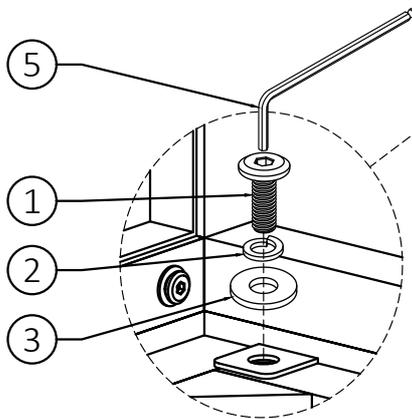
2. Use four Bolts (1), four Lock Washers (2) and four Washers (3) to secure metal frame and Top (A).
