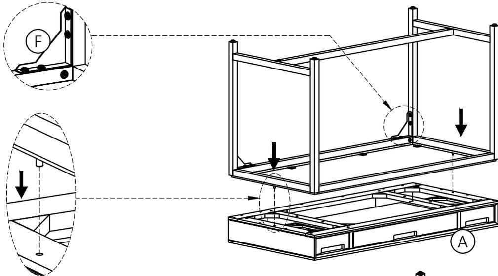
1. Attach the assembled metal frame to Top (A).
