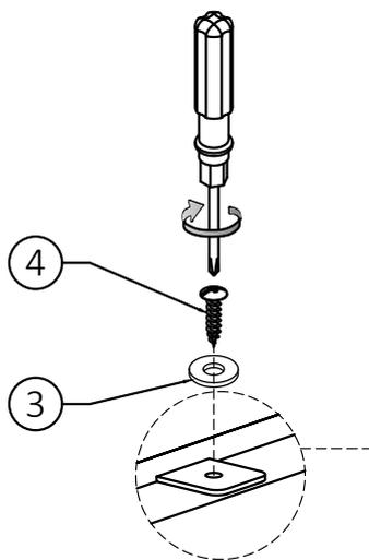
4. Use four Phillips Screws Round Head (4) and four Washers (3) to secure Top (A) and metal frame.
