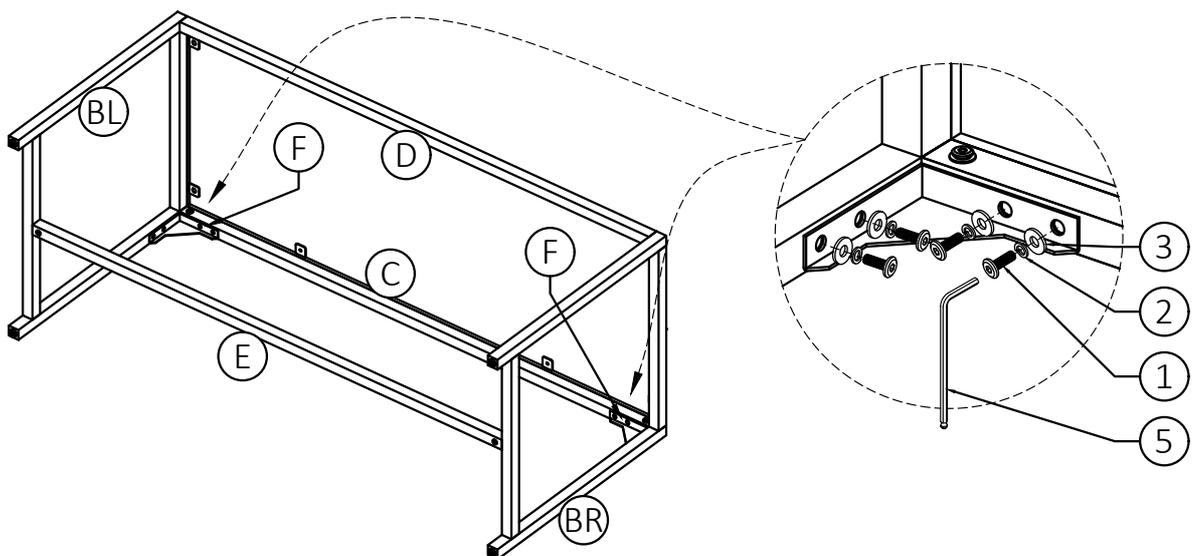
2. Use four Bolts (1), four Lock Washers (2) and four Washers (3) to secure each part (F) with (BL), (BR).
