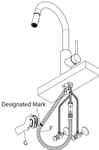
Attach weight (G) on the designated mark on the spray hose (F)
