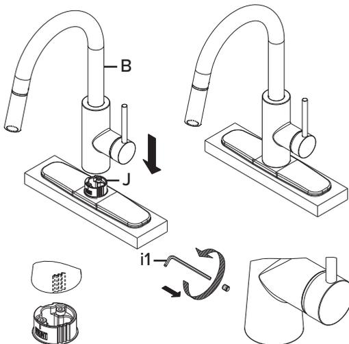
Align arrow on faucet body (B) with arrow on base (J). Attach faucet body (B) to base (J). Secure faucet body (B) by tightening the set screw with 2.5mm hex wrench (i1)
