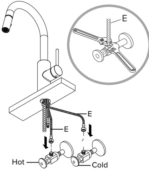
Thread hot & cold waterlines (E) onto angle stops. Tighten with adjustable wrench until snug. Turn on the angle stops and check for leaks (DO NOT TURN FAUCET ON)
