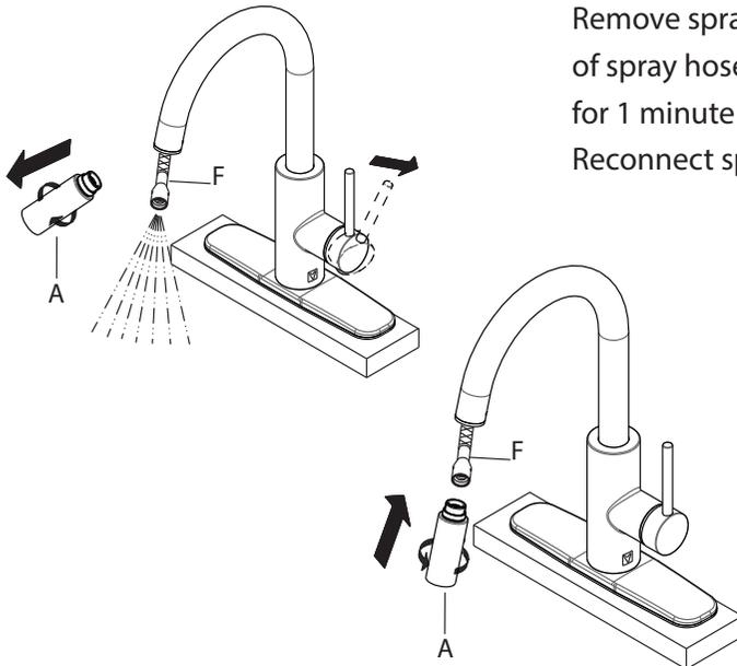
Remove spray head (A). Hold tip of spray hose (F). Turn faucet on for 1 minute to flush any debris. Reconnect spray head (A)
