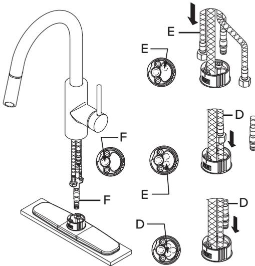
Remove Quick Connect (H) from spray hose (F). Insert spray hose (F) into small hole of base (J). Insert hot & cold waterlines (E) and supply hose (D), one by one, in large hole of base
