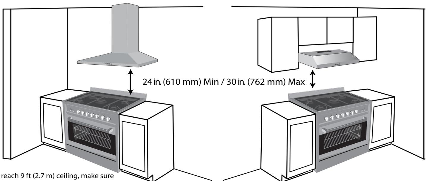
To reach 9 ft (2.7 m) ceiling, make sure range hood is installed at least 33 in. (83.8 cm) from cooking surface.
