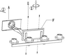
Step 2:Carefully pass outlet box wires through mounting plate (A) Attach back plate (A) to outlet box with mounting screws (C)
