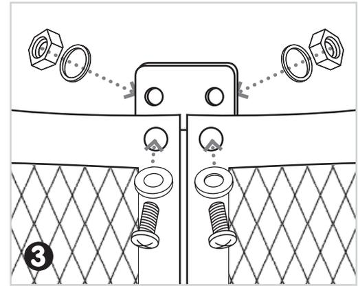
**Hardware Used:** 1x M5x10 Screw/Lock Nut
