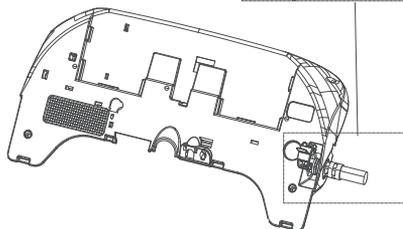
Insert the Metal Snap into the connection between the water supply hose and Inlet connector. (until hearing a "click" sound).
