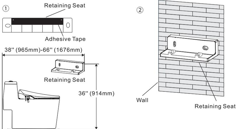
① Select a smooth and even surface to ensure the control holder remains seated.
