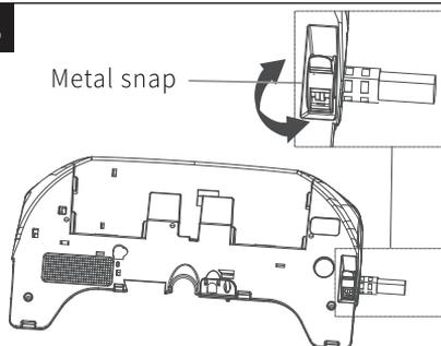
Hold the water supply hose, turn the metal snap slightly, and make sure that there is no obstacle when turning. If there is obstacle when turning, it is indicated that the installation is not correct.
