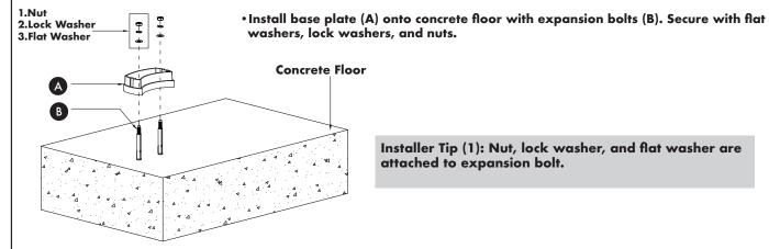
Installer Tip (1): Nut, lock washer, and flat washer are attached to expansion bolt.
