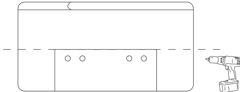
3. Install the hardware using the two provided wall mounts and 4 screws.
