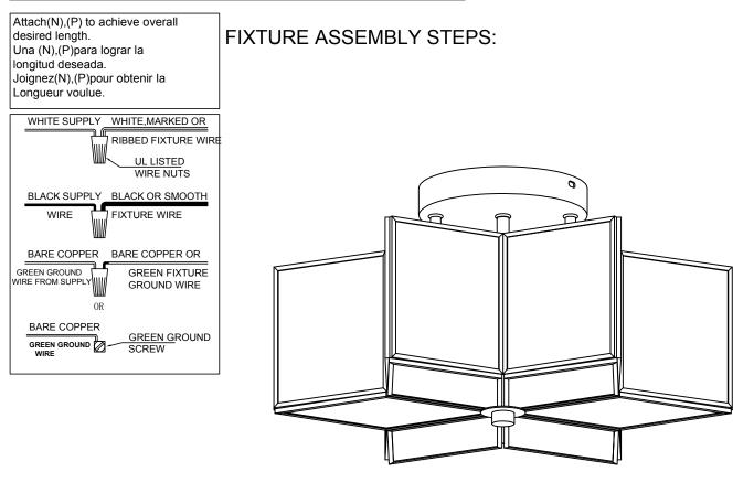
110-120V / 60Hz E26 2\*MAX 60W TYPE A (Do not contain light bulb)
