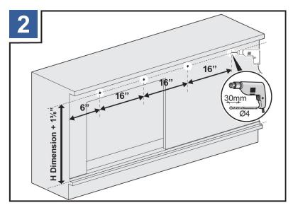
Using a power drill with a 4mm drill bit, drill holes as indicated.
