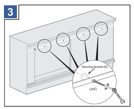
Install the rail, and mounting brackets [E].
