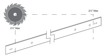
The rail can be trimmed if necessary using a band saw or hacksaw. Use blades suitable for iron or stainless steel depending on your rail.
