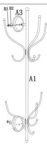
Assemble Metal Plate A3 to Support Rod A1 using Nuts B3 and Flat Washers B2 with a Open Spanner B6 as shown above. Page 3 of 4
