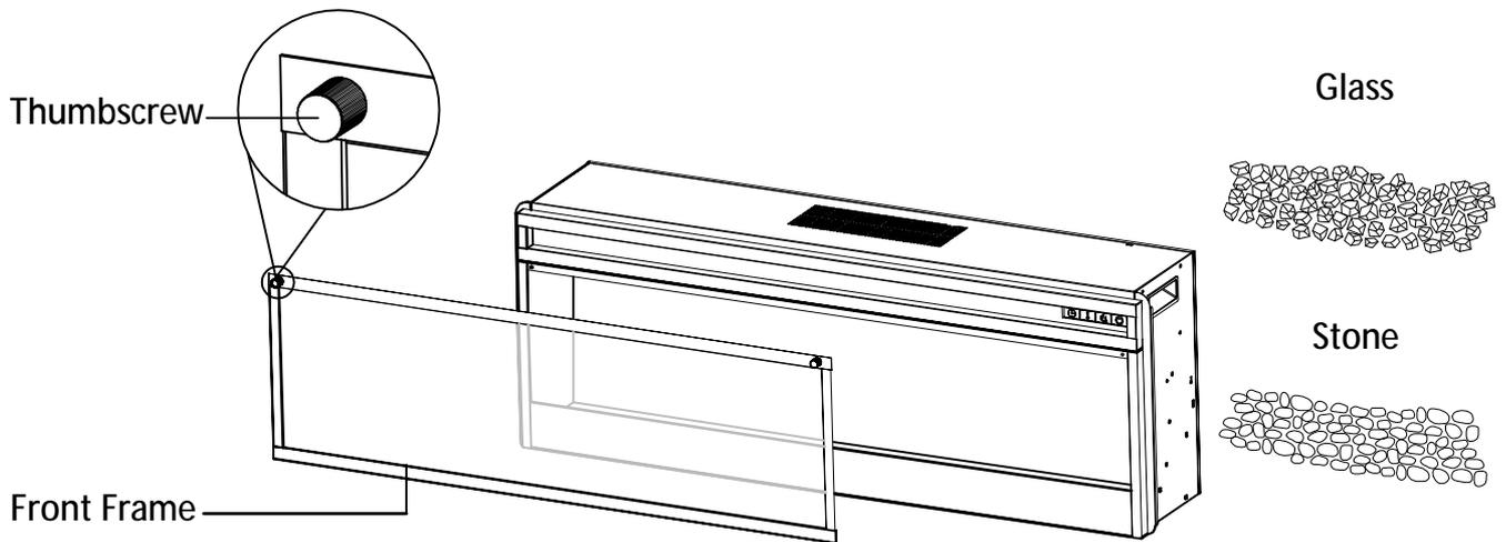
Thumbscrews are attached on front frame and are meant to be permanent and should not be removed.
