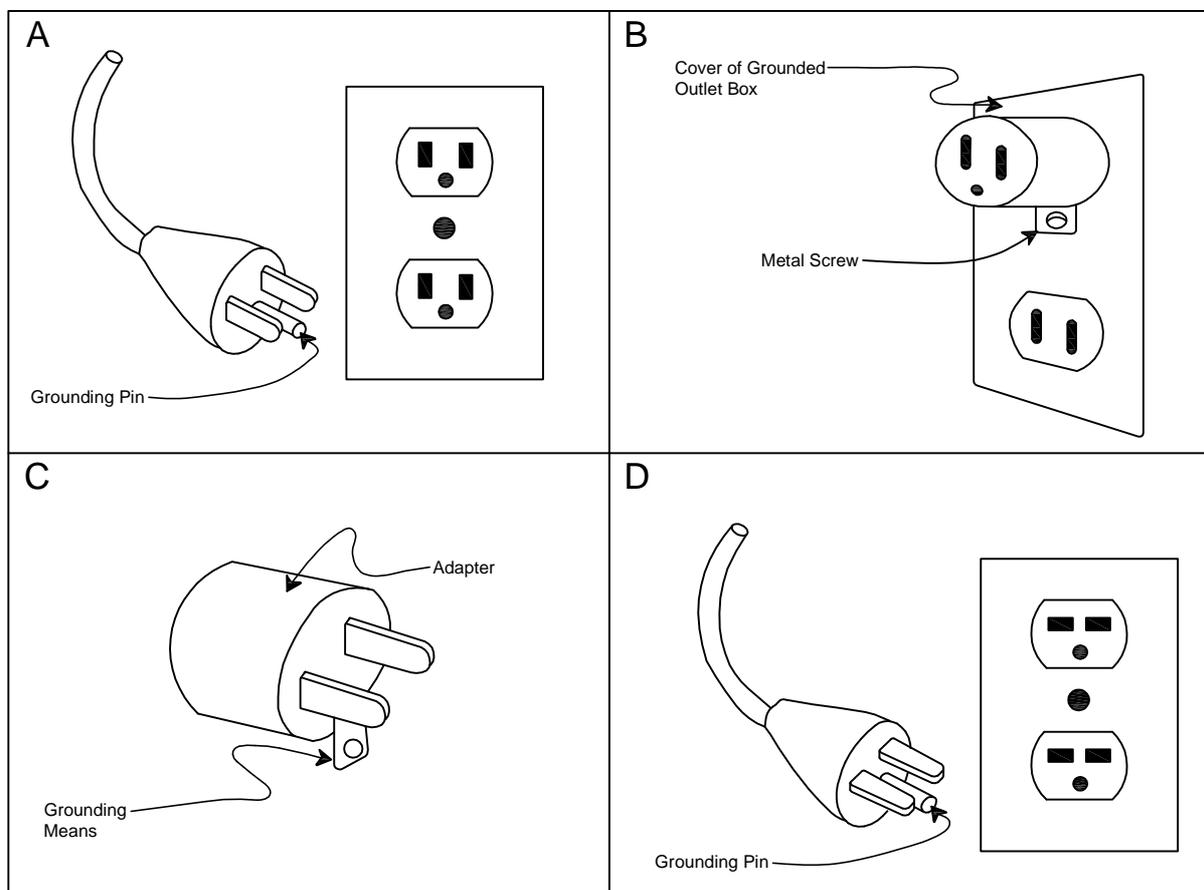
Improper connection of the equipment-grounding conductor can result in a risk of electric shock which may cause serious injury, death or property damage. Check with qualified electrician or service person if you are in doubt as to whether the product is properly grounded. Do not modify the plug provided with the product. If it will not fit the outlet; have a proper outlet installed by qualified electrician.
