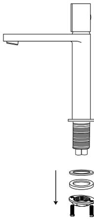
Remove the washer and mounting nut.
