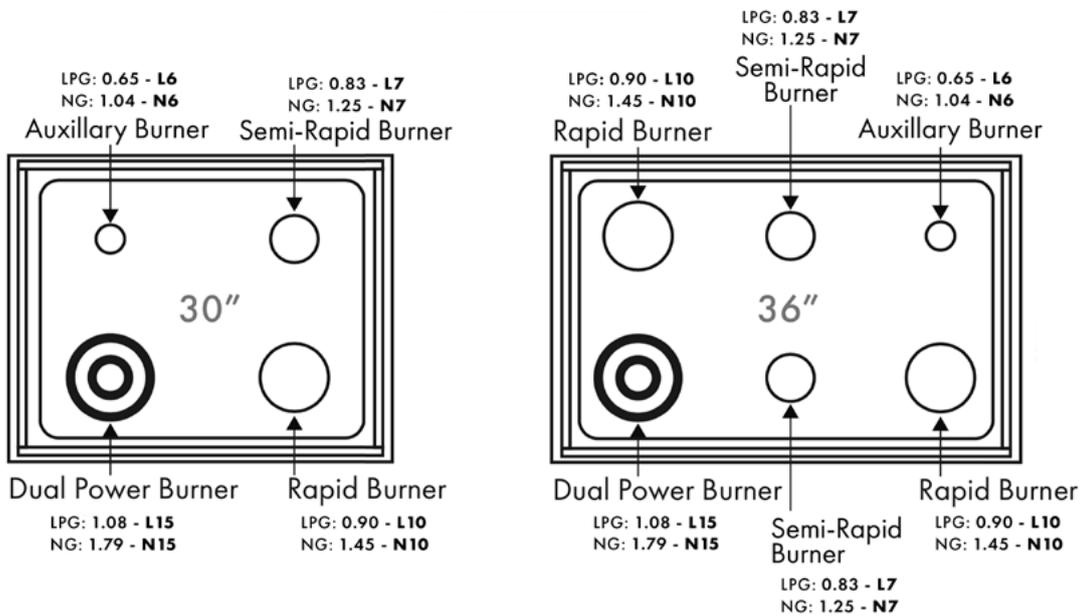
Reference the diagrams below if your drop-in cooktop was manufactured after June 2021. To check, reference the rating label on the underside of the product.
