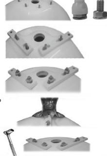
6. While the tub is upside down, take off the plastic caps at each foot location covering screw threads. There will be 1 washer and 1 nut underneath the plastic caps. Take each of these off.
