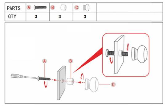
WARNING: To prevent any cracking or breaking of the mirror, please do not overtighten the knobs during installation.
