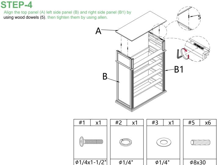
Align back panel (D) top (A) left side panel (B) right side panel (B1) crossbar (F) and bottom panel (C)
