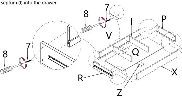
Align bottom drawer panel (Q) drawer side panel (R P) back drawer panel (K) drawer panel (G) and reinforcing panel (Z), then tighten them by using bolt (7)
