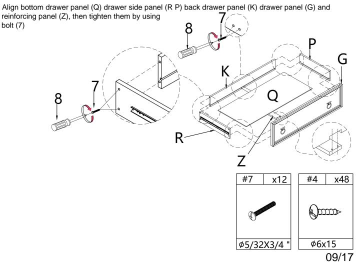
Align bottom drawer panel (Q) drawer side panel (R P) back drawer panel (K) front drawer panel (T) and
