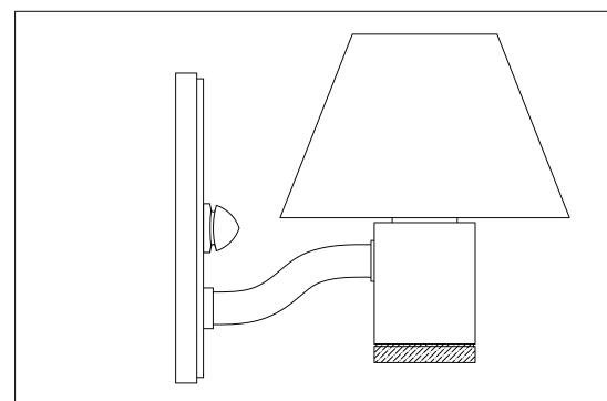
To prevent water intrusion, caulk around back-plate where fixture meets the wall using outdoor silicone sealant. Leave a small gap at the bottom to allow moisture to exit.
