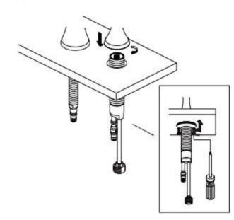
fitting to lock, pull down to check for secure connection. NOTE: To install the quick fittings, follow these simple steps:
