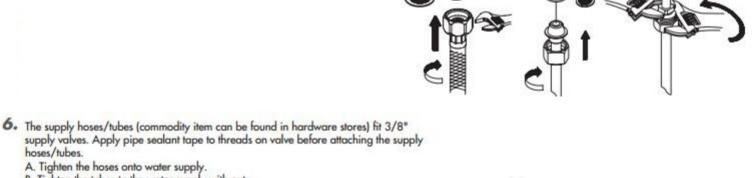
A. Tighten the hoses onto water supply. B. Tighten the tubes to the water supply with nut.
