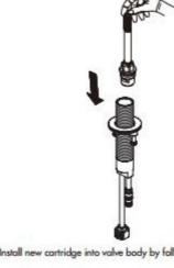
4. Install new cartridge into valve body by following step 1,2 and 3 reversely.
