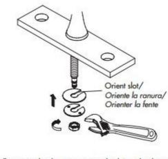
2. Install mounting hardware onto spout shank in order shown. Orient spout to center of sink, then tighten locknut. Important: Orient slot in mounting washer to rear of spout to allow lift rod for drain to pass through.
