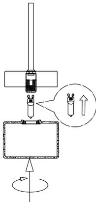
Insert G9 shielded bulb max 25W to the socket. Bulb is not supplied.
