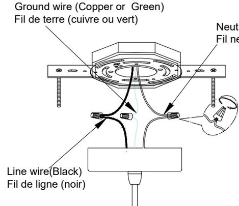
Connect the GROUND WIRE from junction box to GROUND (or GREEN) wire from fixture with a wire nut. Connect the NEUTRAL WIRE from junction box to NEUTRAL (WHITE) wire from fixture with a wire nut. Connect the LINE WIRE from junction box to LINE (BLACK) wire from fixture with a wire nut.
