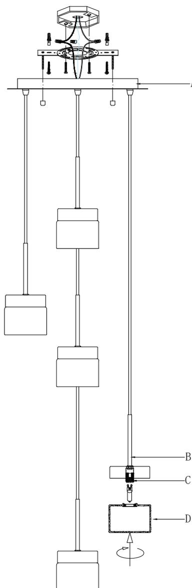
Before installation to ceiling, adjust fixtures to desired length.
