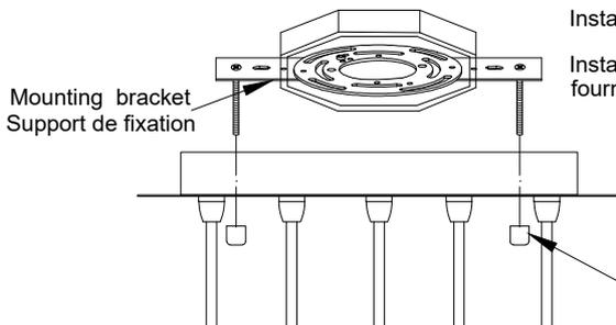
Install the canopy to mounting bracket with cap nuts provided.
