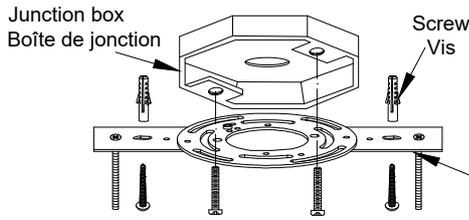
Attach mounting plate to junction box with screws provided.
