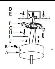
**Step 3:**Punch the hole and install the Wall plug (E) to the ceiling. Fix the mounting bracket (F) to the outlet box with tapping screw (H) and mounting screw (J).
