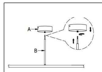
**Step 1:**Run the main line through canopy (A), then tighten the canopy (A) and the lamp body (B).
