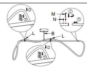
**Step 5.** One end of the support(L) is stuck in the lamp body (B) and the other end is stuck in the hose. Hose wrap around the lamp body (B) and secure it with allen wrench (M) and hex screw(N).
