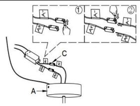
**Step 2:**In canopy (A), the main line and the transformer according to the corresponding letters of the label in turn with connectors (C) connection.
