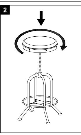
**Step 1**To lift up, turn the cushion seat counter-clockwise.
