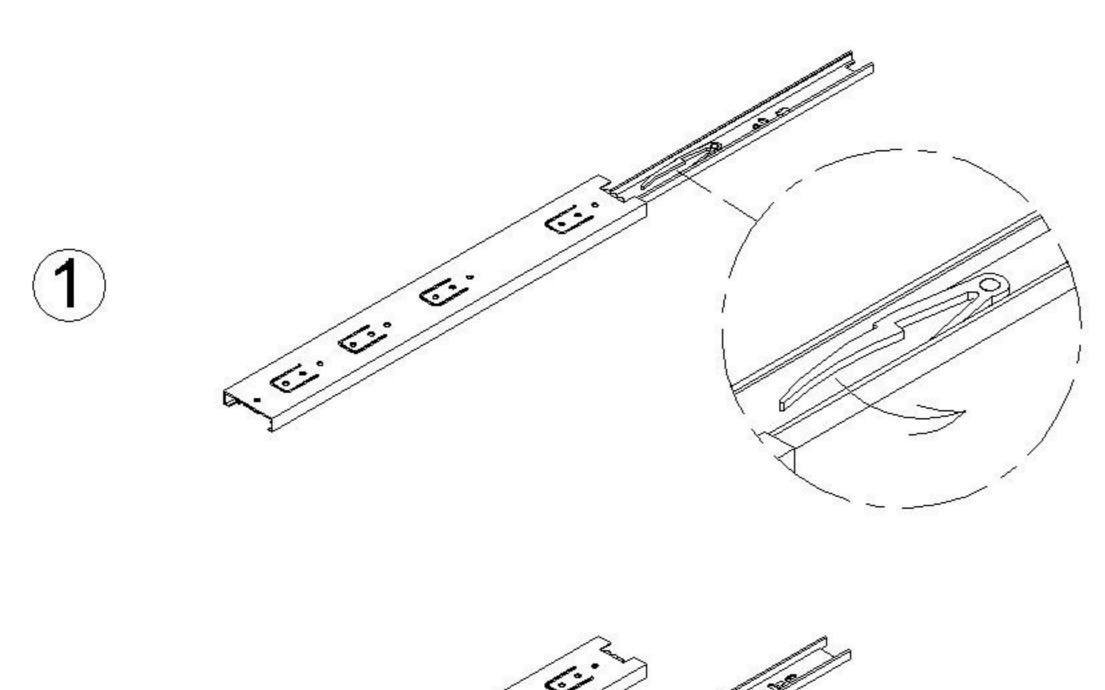
Disassemble the glides to tighten on panel. Glides will be disassembled in 2 parts, 1 part to fix on side panel and the other part to fix on drawer side.
