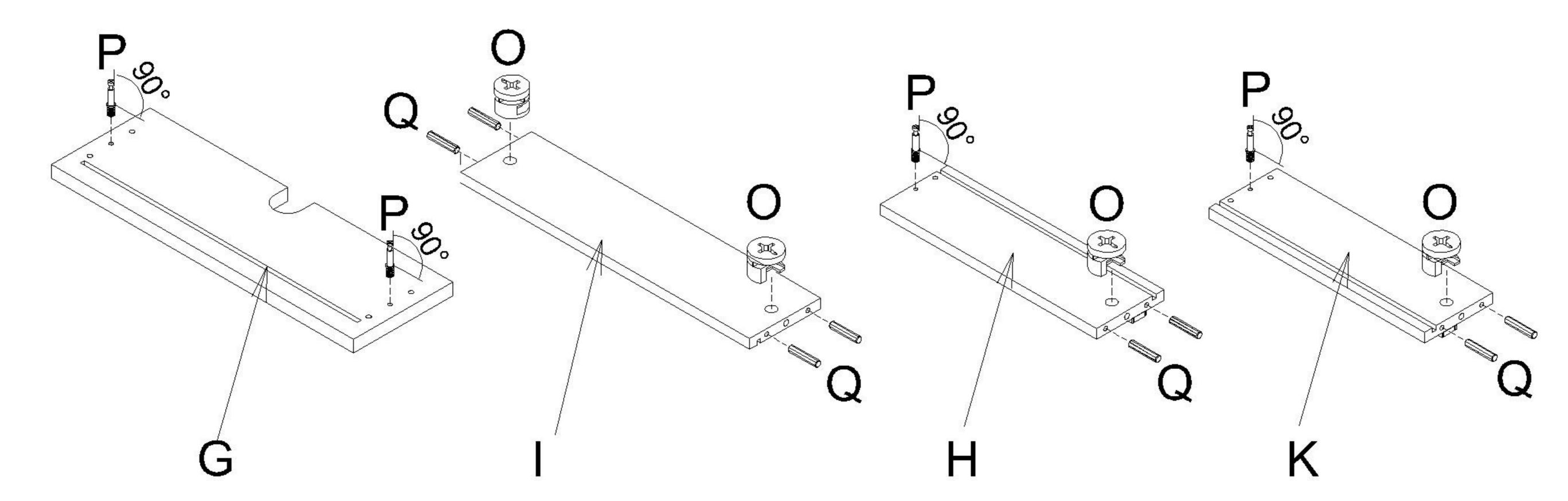
Attach Left & Right Drawer Side (H & K) to Drawer Back (I) and secure with Cam Lock (O). Use Cam Lock Cover (R) to cover Cam Lock (O).
