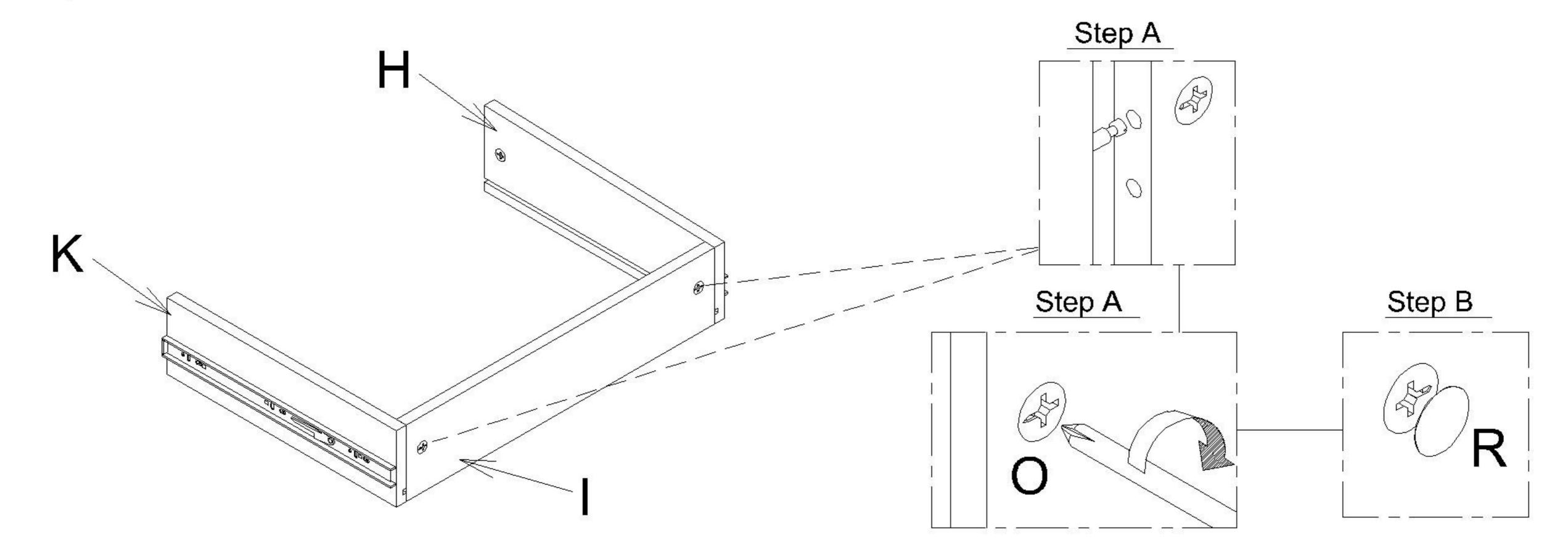
Slot in Drawer Base (J) in corresponding grooves. Attach Drawer Front (G) to Drawer Box and secure with Cam Lock (O). Use Cam Lock Cover (R) to cover Cam Lock (O).
