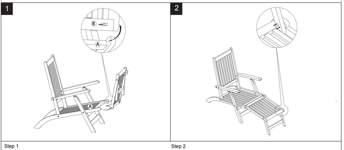
(A) attached with (B) when the lock pull up which is followed up the arrow.
