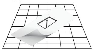
3. Determine the location of the drainpipe on the floor by taking measurements of the drain and waste location underneath the unit. Clean the drain hole area in preparation of setting the drain. The area should be dry & free from any debris.
