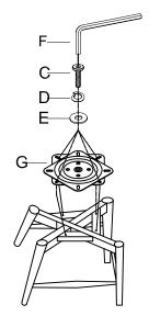
Take the allen key, and turn the bolts until the legs are secure. DO NOT TIGHTEN COMPLETELY. Stop when you feel you are adding force to tighten the bolt.
