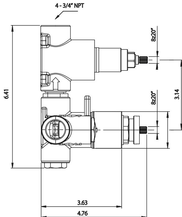
TVH.4420 | 3/4" Thermostatic Valve With 2-Way Diverter & Integrated Volume Control
