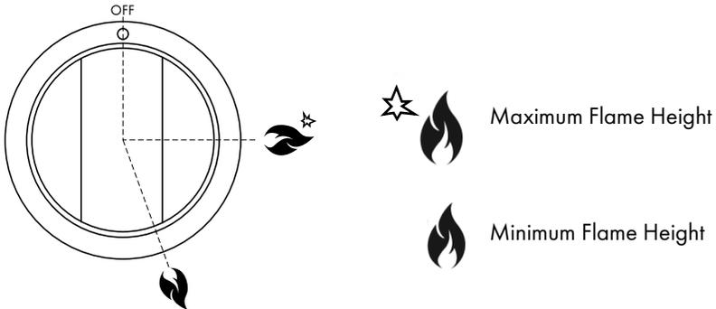
Maximum temperature setting/recommended control knob position for burner ignition.
