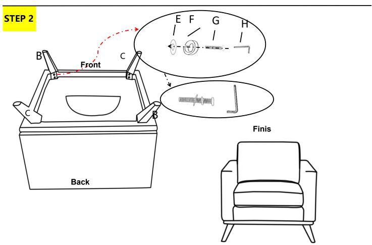
NOTE:DO NOT TIGHTEN ANY BOLTS UNTIL ALL BOLTS HAVE BEEN STARTED!
