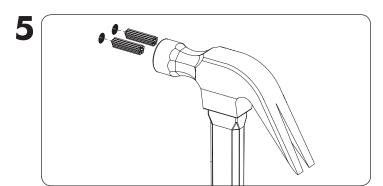
Insert provided anchors if mounting into drywall. Anchors not necessary if mounting into wood studs.
