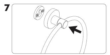
Place the towel ring over the mounting plate with the set screw on the bottom.
