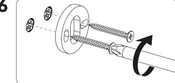
Install the mounting plate with the provided screws.
