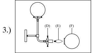
step3: Loosen the lock screws (D). Install E12 bub(E) and attach glass (F). Secure glass (F) by tightening lock screws (D).
