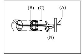
step2: Wire fixture to wires in outlet box. Copper wire is for Ground. Attach wall sconce to mounting bracket and tighten ball nuts (A) so fixture meets wall.
