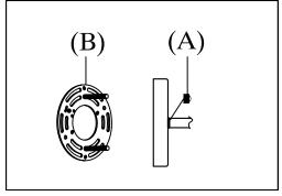
step1: Remove mounting bracket (B) from fixture and install to electrical box using mounting screws (C).
