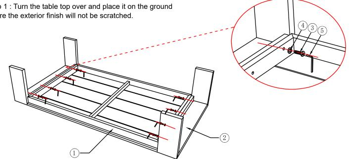
Step 2 : Align the screw holes of the table legs with the screw holes of the table top, insert flat washers(4) and screws(3) into each hole, once the screws are in place, tighten the screw until firmly attached with the wrench provided.
