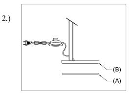
Step 2: Adhere the felt pad (A) to the bottom of the weight (B).
