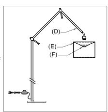
Step 3: Remove the socket ring (F) from fixture (D). Attach shade (E) and secure using socket ring (F).
