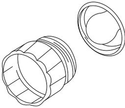
To replace the G9 halogen light bulbs (2) located at the upper left and right corners of the SGR30, SGR36, and SGR48 large oven, unscrew the protection cap that projects out inside the oven. The SGR48 small oven has 1 bulb.
