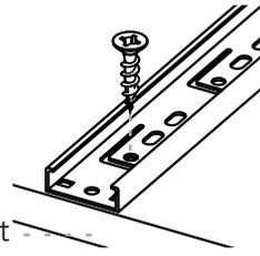
Take the bigger part of the slide and place it over the panel. The plastic stop should go towards the back.
