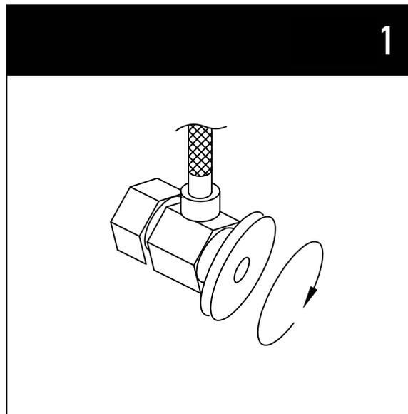
1. Shut off water supply. Remove old faucet and flexible hoses. Clean sink surface in preparation for the new faucet. Flush water connection at home to make sure no debris is stuck in the line.
