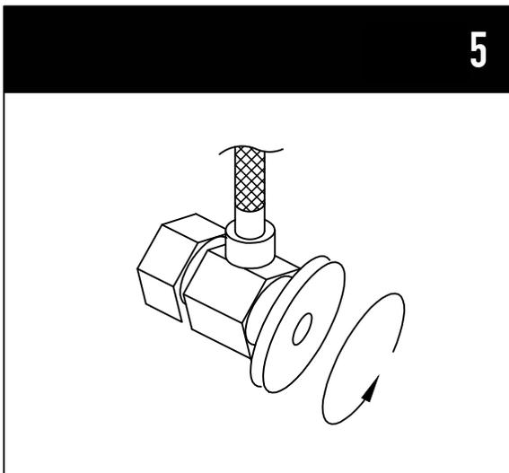
5. After installation is complete, remove the aerator. Turn on the water supply valves and allow both hot and cold water to run at least one minute each. While water is running, check for leaks, especially at hook-ups to supply lines. Tightening nuts slightly will stop any minor leaks.
