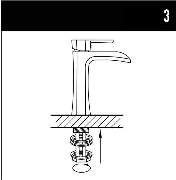
3. Place new faucet in the position on the sink. From under the sink, put rubber washer, metal washer and thread nut onto the pin. Tighten nut.
