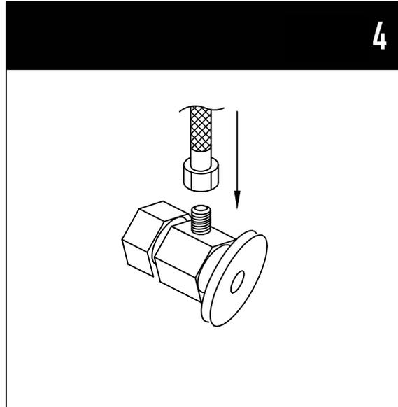
4. Connect female end of flexible hoses to the cold and hot water supply.
