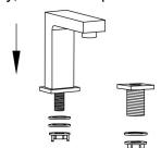
4. Three switches main body from the bottom up through the table, fasten the screw and handle by hexagonal tool after alignment to the base. Finally fasten the nut.
