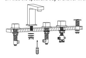
6. Pulling pipe connect with the connector A through the shower holder. Gravity ball fixed on the top of the pull out pipe. Water nozzle connect to the conversion B, hot and cold switch connect with connector C and D respectively and finally contact to the hot and cold water hose.
