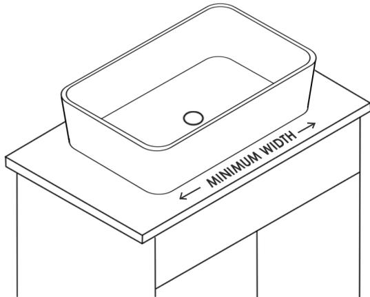
Position sink vessel on the installation surface and confirm vessel size is correct and don't interfere with faucet
