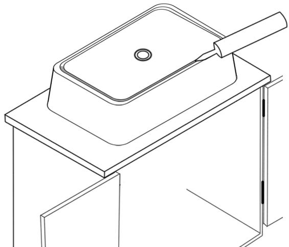
When sink is ready to be installed, put sink up side down and apply a bead of silicone on the outer channel of the sink vessel, alternative use plumber's putty cord.
