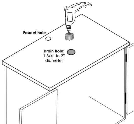
Drill drain hole on the countertop, the size of the countertop drain hole recommended is 1-3/4 inches to 2 inches.
