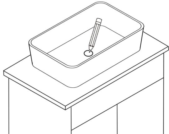
If drain hole has not been made, mark the drain hole location on the countertop.
