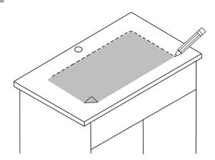
Place cut-out template in desired position on countertop locating center of the bowl over cabinet.
