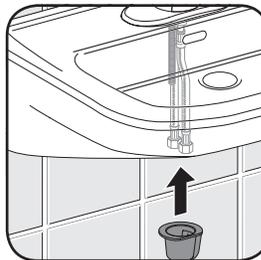
3. Mount bracket from underneath. Place hoses through large opening and mounting rod through small opening. Make sure flange sits securely against surface.
