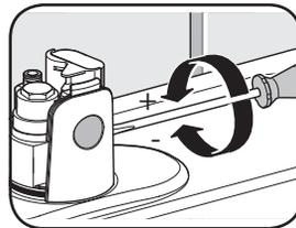
3. Adjust internal mixer with screwdriver
