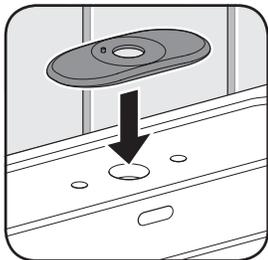
1. Mount cover plate if required. Plumber's putty is recommended to seal cover plate to the sink. Security pin must be located on the left side.
