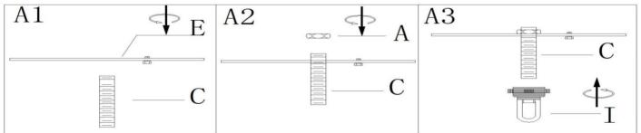
Step A1: Thread the single bar(E) onto nipple (C),
