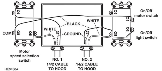
Install 2 included rocker switches at a convenient place for the user. Use two 14/2 cable to wire the switch box to the range hood (see diagram above).
