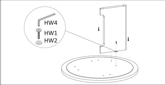
STEP 2: Carefully place the marble top (A) on a soft surface. Align the screw holes on the marble top to the screw holes on the assembled legs. Use the allen key (HW4) to screw in the jcb bolts (HW1) through the flat washers (HW2) to attach the legs.
