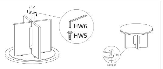
STEP 3: Attach the remaining legs to the marble top (A) as shown. make sure there | STEP 4: Attach the base assembly plate (C) to the bottom of the legs by using the allen key (HW6) to screw in the csk bolts (HW5) as shown. adjust the levelers as needed. product is now ready for use.
