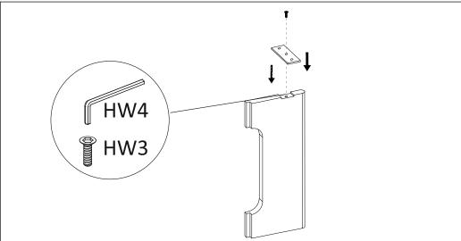
**STEP 1:** Place the leg upright and align the screw holes on the top assembly plate (D) to the screw holes on the leg (B). use the allen key (HW4) to screw in the csk bolts (HW3) as shown. repeat this process for the remaining legs.
